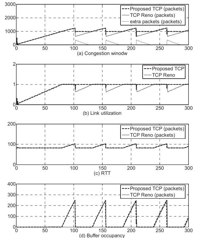
**Fig.3** Comparison between the proposed TCP scheme and TCP Reno.
