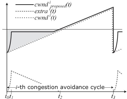
Fig. 2 The congestion window evolution and extra transmitted packets of the proposed TCP scheme during one congestion avoidance cycle.
