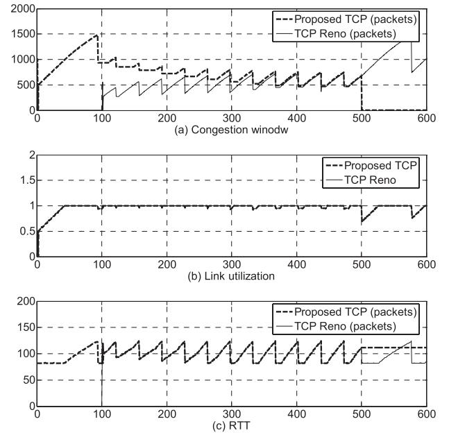
**Fig. 5** Comparison of the proposed TCP scheme and TCP Reno.
