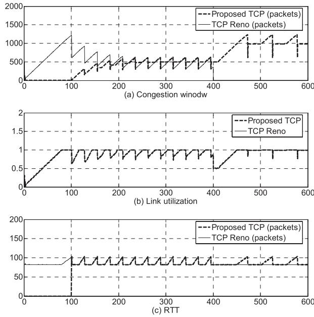
**Fig. 4** Comparison of the proposed TCP scheme and TCP Reno.
