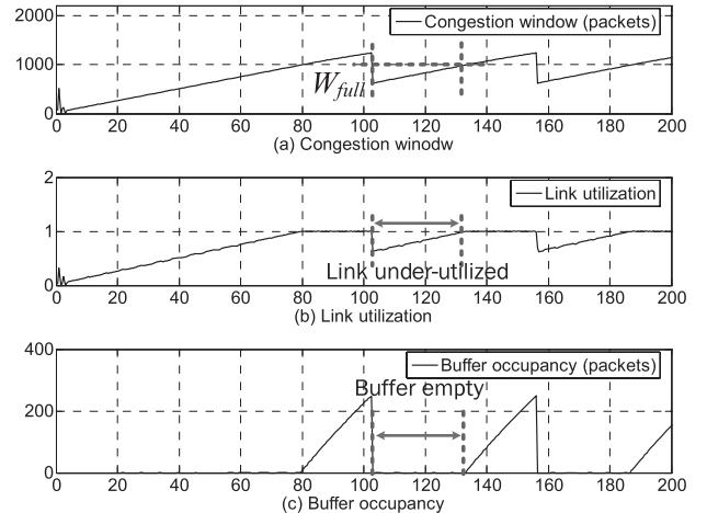
Fig. 1 TCP Reno operation in an under-buffered link.
