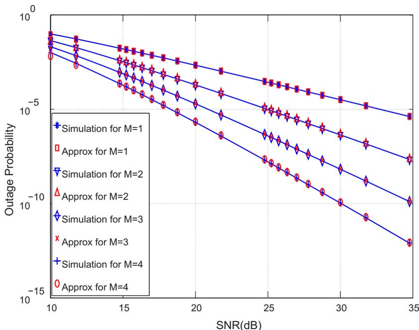
**Fig. 3** Outage probability for the ARC scheme
