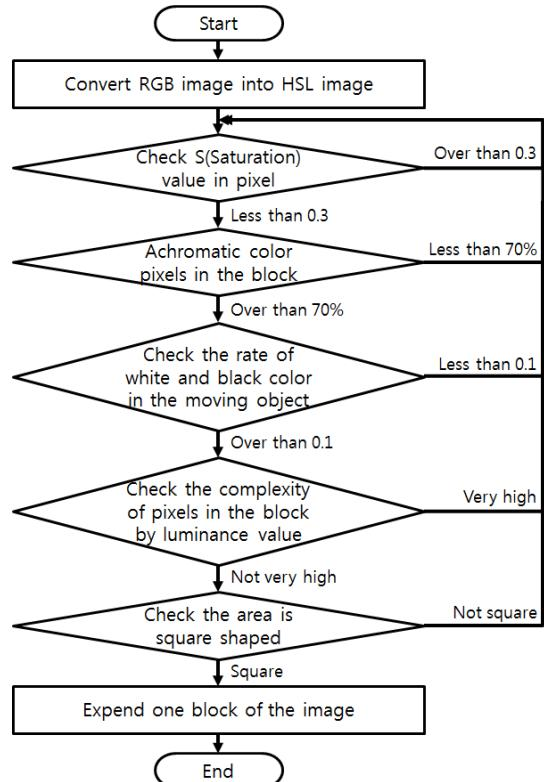
Figure 7. Flowchart of Extracting Barcode from Object Image
