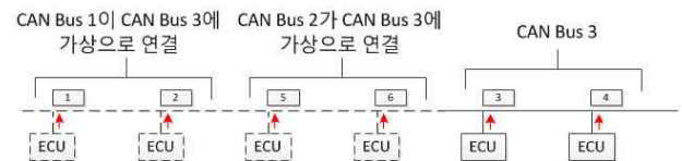
Fig. 3 Virtual connection of Source CAN Bus and destination CAN Bus
